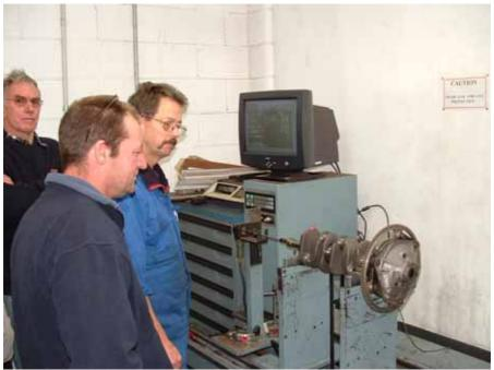
Balancing a Mini crankshaft & flywheel
